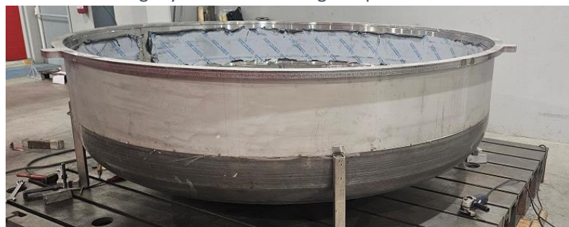
Above: The bottom segment of the Cryostat during manufacturing. Credit: Dal Ben
